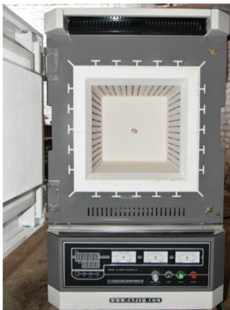
Figure:3. Temperature-controlled electric furnace.
